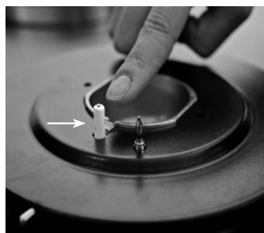
Electric spark ignition
