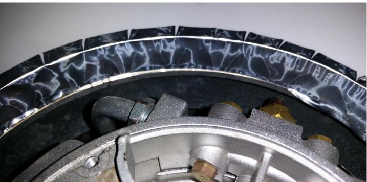
In the regulations of Corian they state that it is mendatory that cut-outs have a fillet of atleast 1.5mm. It is also required to apply aluminum conductive tape around the cut-out. (See chapter 7 of the Corian manual.) You can find these requirements in our processing manual as well. (We took the manuals of some very big solid surface suppliers and used them as a base for our manual.)
