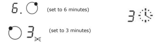
2. When cooking timer expires, the corresponding cooking zone will switch off automatically.
